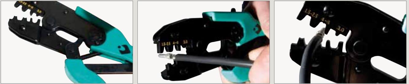
Example of use of the IS3161 crimper for Cabur Solar connectors.
